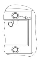
Fig.6 Replacing a light bulb
